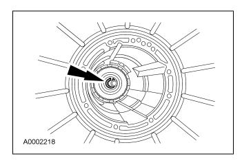
24. **NOTE:** Install the output shaft sleeve with the cone facing up. This sleeve will snap into place when correctly installed.
